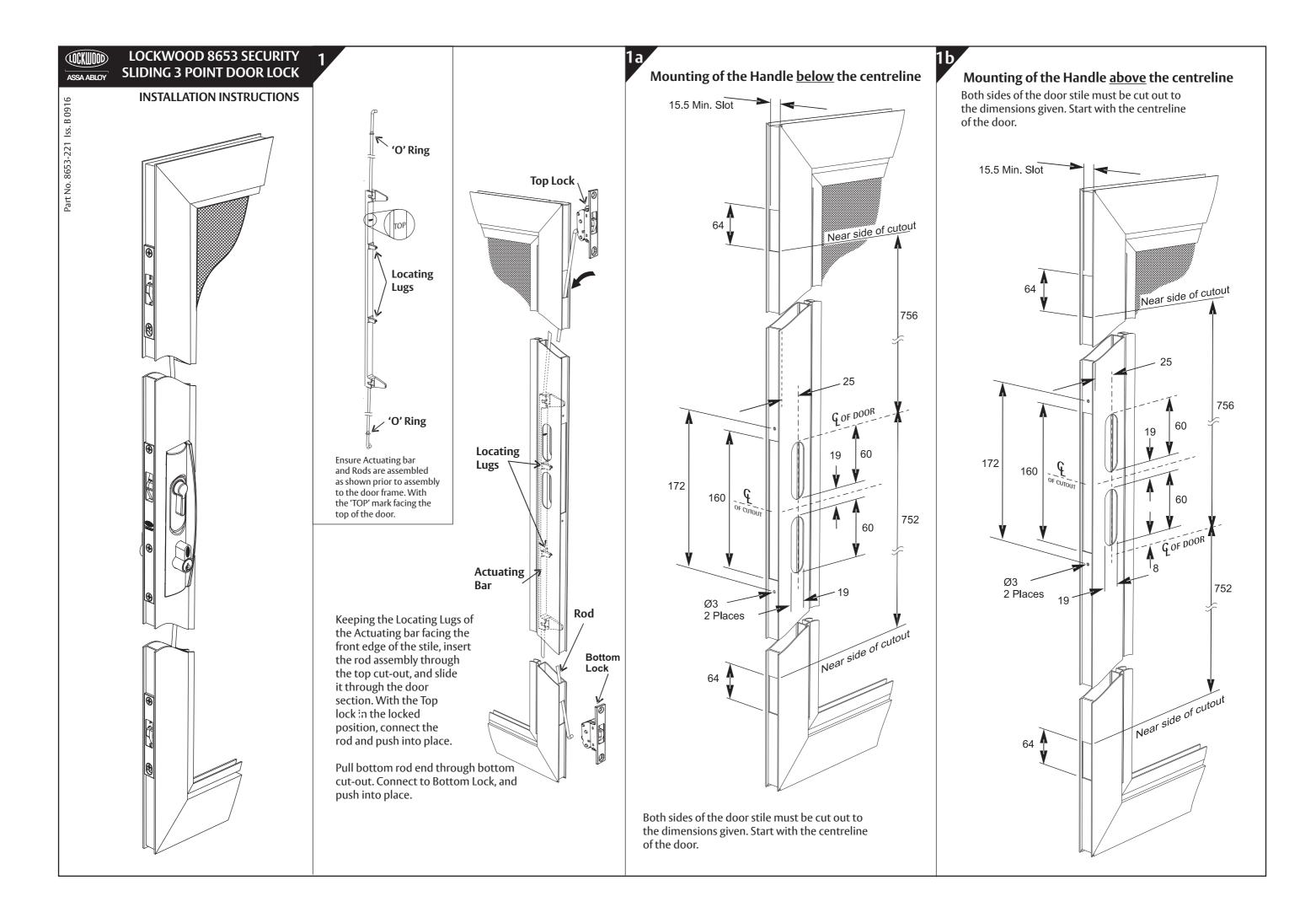
After ascertaining the handing configuration required, simply click the desired handle plates together and install the operating levers and external restrictor plate as required. Then secure the furniture plates to the door section using the two 25mm screws & plugs supplied.
